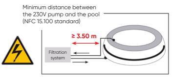
You must use a socket fitted with a 30mA differential circuit breaker. <u>More details on</u> pages 18 and 19 of this leaflet.
