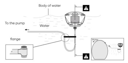
As it floats freely on the water, this floating skimmer has the advantage of automatically adjusting itself in relation to the body of water.
