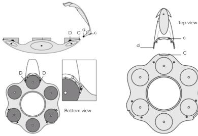
Note: check that the clips (d) are properly engaged in the notches (D).
